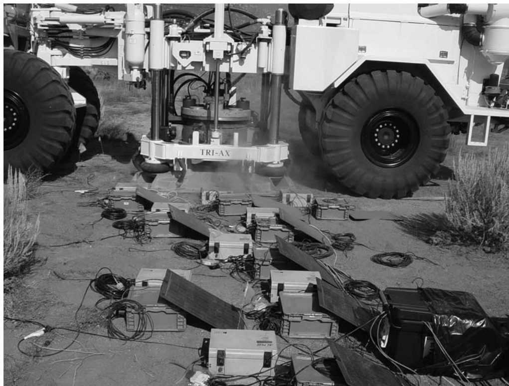
Figure 1. Photo of the experiment. Shown is the NEES mobile shaker truck, T-Rex. Adjacent to T-Rex is the accelerometer array installed to record the induced high-strain seismic waves. Each three-component K2 accelerometer has an external battery and solar panel attached.
