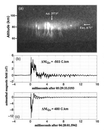
**Figure 2.** (a) Enlarged  $(6^{\circ} \times 4^{\circ})$  image of the negative event at 05:29:33.522 UT showing a well developed spritehalo with streamers. (b) The ELF/VLF azimuthal magnetic field (B $\varphi$ ) waveform associated with this event. (c) The B $\varphi$  waveform of a sprite-halo (Figure 3c) produced by a positive CG of similar  $\Delta M_{Qv}$ .
