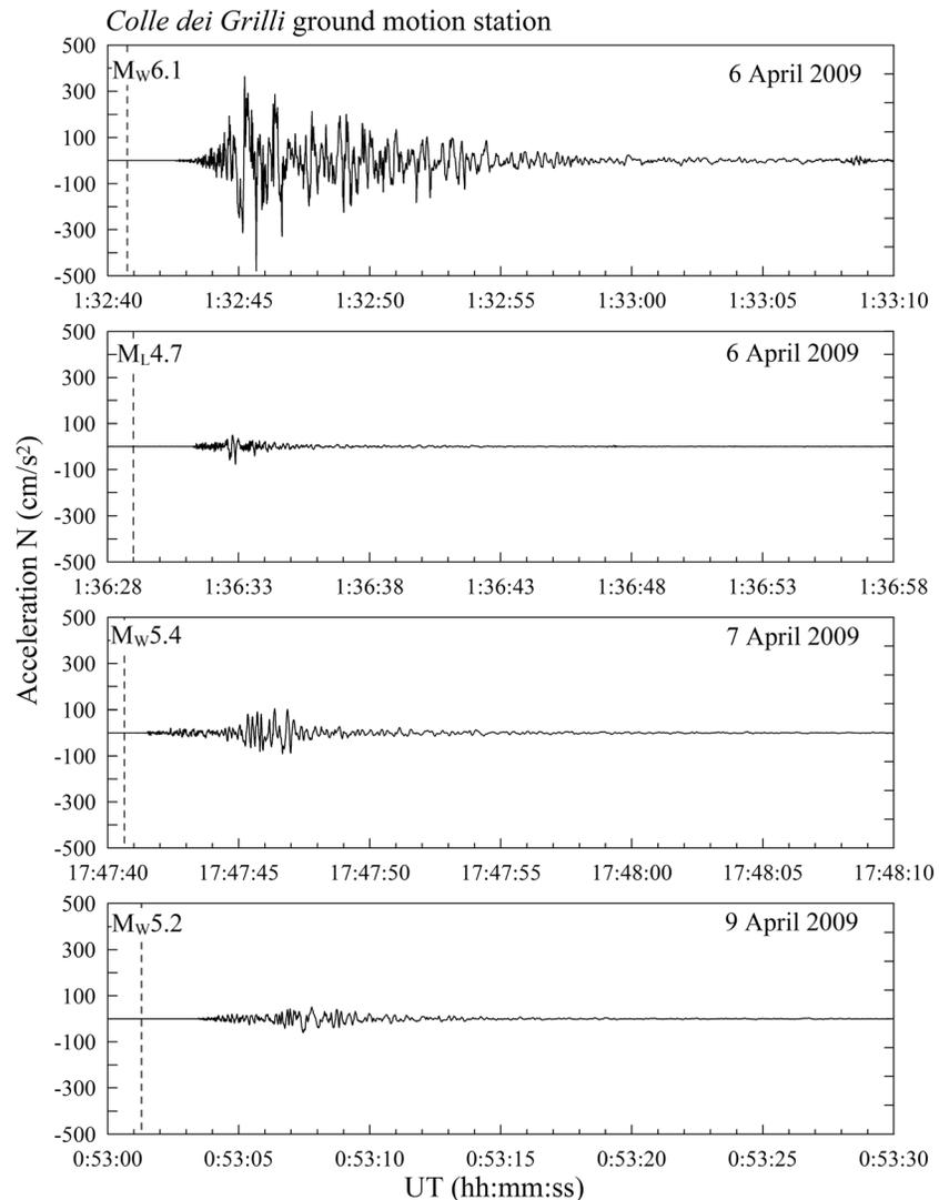
**Figure 4.** The  $N$  component of the ground acceleration from the strong motion station of Colle dei Grilli in correspondence with the 6 April  $M_w6.1$  main shock and  $M_L4.7$  aftershock, and the two largest aftershocks of 7 and 9 April.
