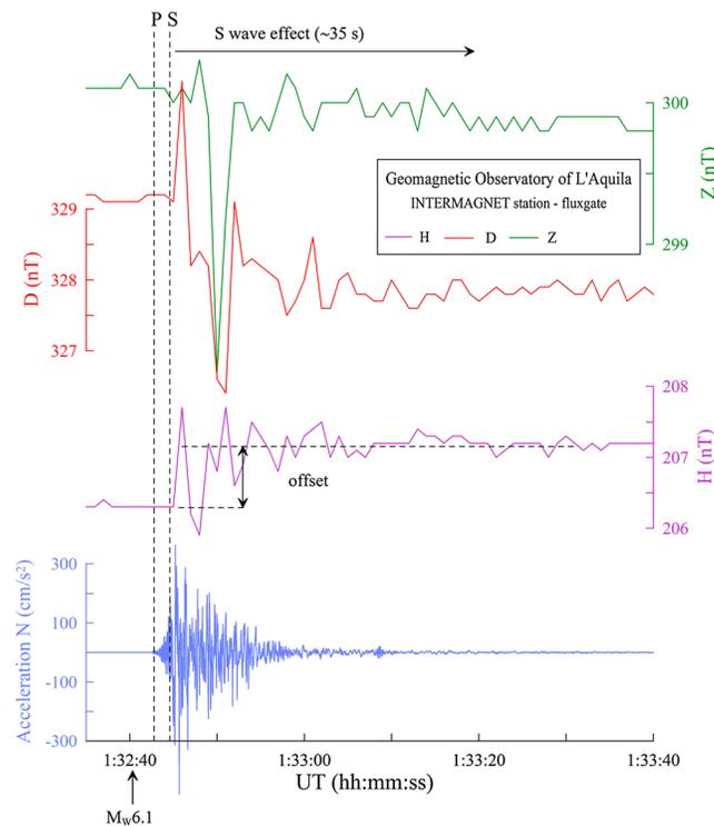
**Figure 2.** Magnetic field  $H$ ,  $D$ , and  $Z$  components from the fluxgate of the INTERMAGNET station at the Geomagnetic Observatory of L'Aquila. The  $N$  component of the ground acceleration from the station of Colle dei Grilli is shown as well.  $P$  and  $S$  are the arrival times in the observatory of the  $P$  wave and  $S$  wave of the  $M_w6.1$  main shock, respectively.
