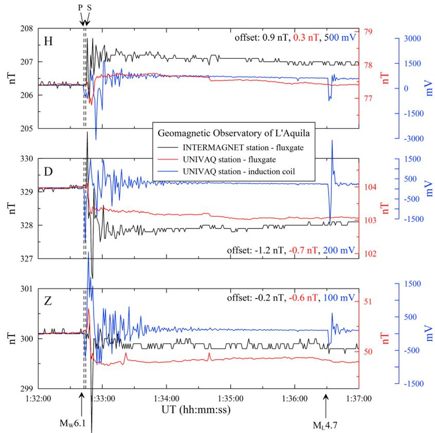
**Figure 3.** Magnetic field  $H$ ,  $D$ , and  $Z$  components from the fluxgate of the INTERMAGNET station and from the fluxgate and induction magnetometers of the UNIVAQ station at the Geomagnetic Observatory of L'Aquila.  $P$  and  $S$  are the arrival times in the observatory of the  $P$  wave and  $S$  wave of the  $M_w$ 6.1 main shock, respectively.
