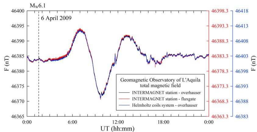
**Figure 5.** Total magnetic field at the Geomagnetic Observatory of L'Aquila during 6 April 2009 from the two overhausers and that calculated from the fluxgate components. The fixed offset between the total field records ( $\Delta F_{\text{INTERMAGNET}} = 1.7 \text{ nT}$ ,  $\Delta F_{\text{overhauser}} = -18 \text{ nT}$ ) is related to the distance between the sensors.
