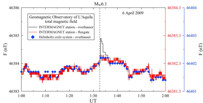
**Figure 6.** Enlarged view of Figure 5 from 01:00 to 02:00 UT. Total field data from fluxgate measurements during the shaking effect (from 01:32:44 to 01:33:19 UT) are not shown. The transient effect in the total magnetic field data from the INTERMAGNET overhauser is not present in the total field calculated from the INTERMAGNET fluxgate components, as well as in the total field from the second overhauser. See text for details.
