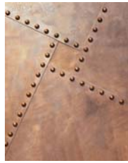
Rivets on skin surface add significantly to total drag at supersonic speeds
