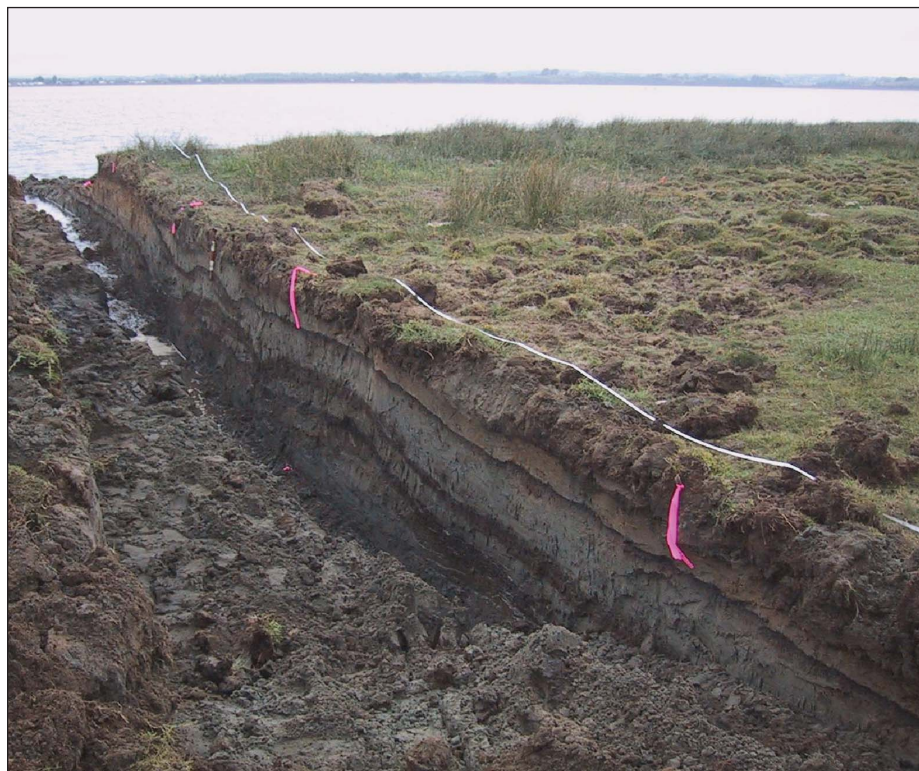
Fig. 1. Sediments fringing an estuary in southern Chile contain deposits of the tsunami generated by the great M9.5 earthquake of 1960 and earlier tsunamis accompanying great earthquakes of the past millennia. Dark layers are organic-rich A horizons of soils buried by light-colored sheets of tsunami-deposited sand. The pink tape markers lie at five-meter intervals. Through study of similar stratigraphic records on the coasts of the Indian Ocean and elsewhere, the recurrence of large earthquakes and the heights, velocities, and inland extent of their destructive tsunamis can be studied.
