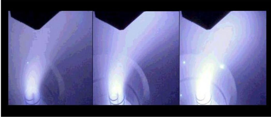
**FIGURE 4.** Time evolution of the plasma production and motion of the magnetic field lines during a 800 msec shot in 500 G magnetic field and 2 mTorr of argon with the frames being separated by 250 msec.
