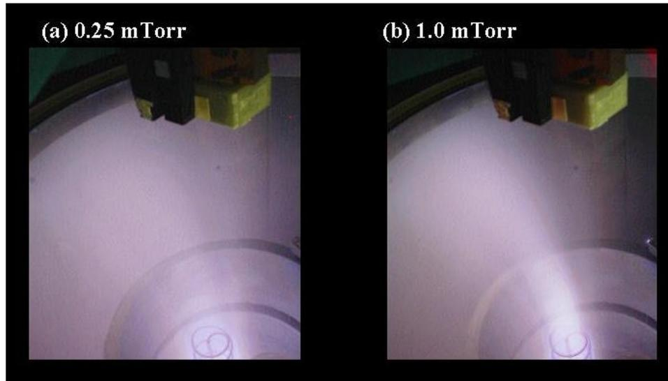
**FIGURE 3.** Plasma production in argon using a bare wire antenna for a field strength of 350 Gauss. Left hand side shows the emissions near the minimum neutral pressure required for breakdown to occur.
