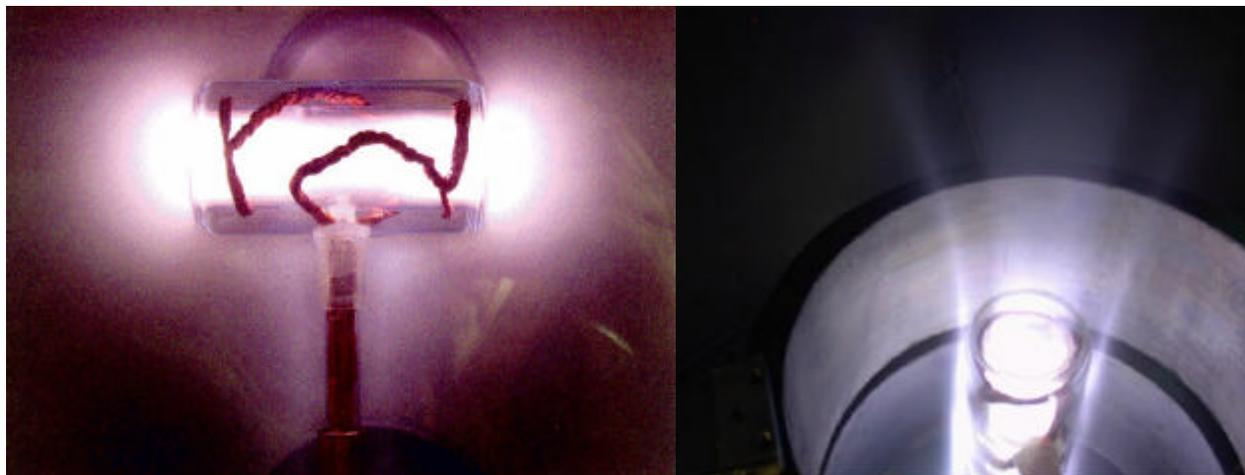
**FIGURE 2.** The production of plasma with no magnetic field (left hand side) and at 350 G magnetic field (right hand side).
