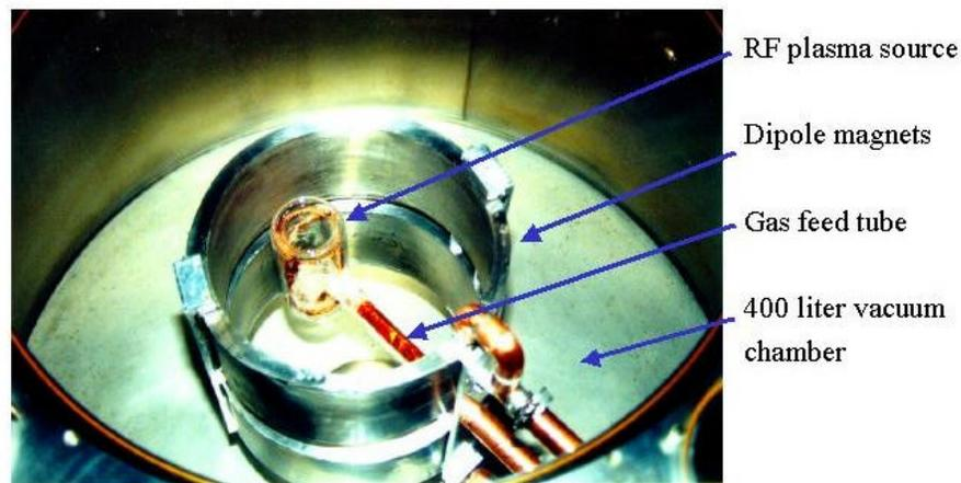
**FIGURE 1.** The M2P2 prototype in a small (1m) vacuum chamber at the University of Washington.
