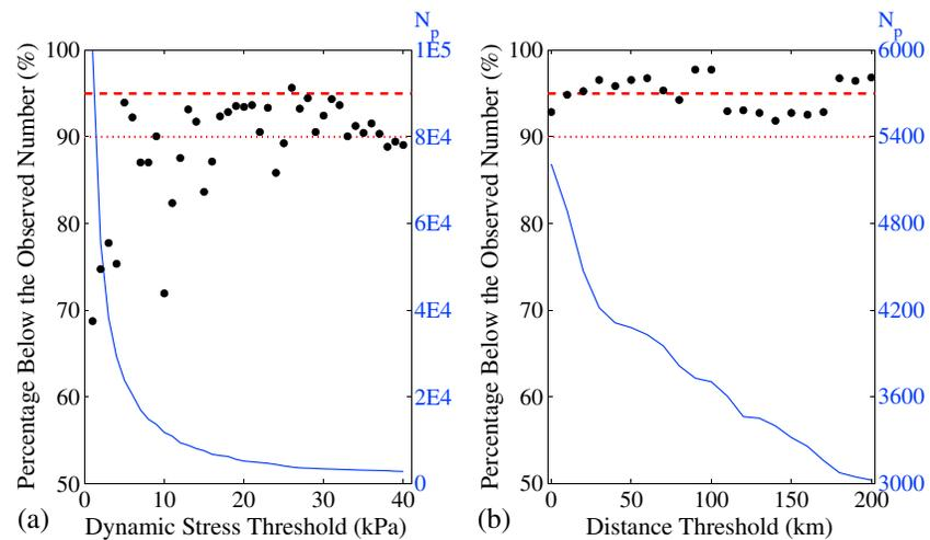
**Figure 4.** (a) Monte Carlo test results using different dynamic stress thresholds. Black circles show the fraction of the distribution of counts derived with randomized perturbation times below the observed count. The blue curve shows the number of perturbations ( $N_p$ ) for each dynamic stress threshold. The horizontal red dashed and dotted lines mark the 95% and 90% levels, respectively. (b) Similar plot as in Figure 4a using different distance thresholds.
