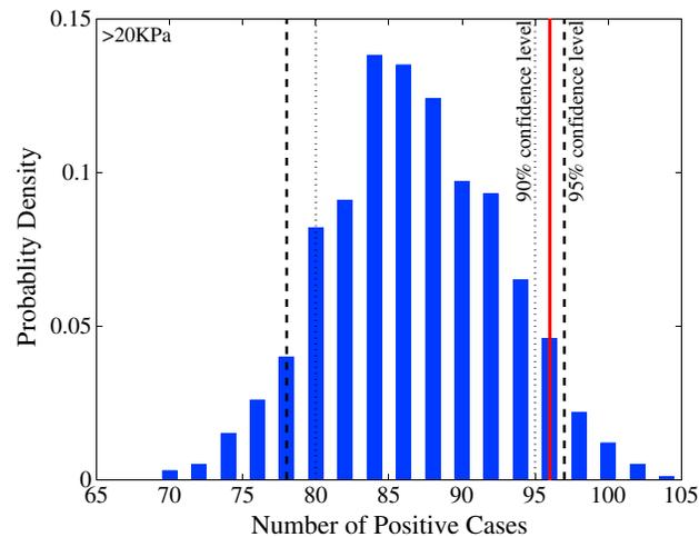
**Figure 3.** Monte Carlo results for a dynamic stress perturbation threshold of 20 kPa. The blue bars show probability distribution function of the 1000 counts of perturbations that occur within shortened recurrence intervals, derived using perturbations with their times randomized. The vertical black dashed and dotted lines show the 5%–95% and 10%–90% levels, respectively. The vertical red line marks the observed count.
