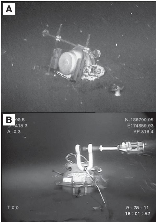
**Figure 2.** Photos of ocean-bottom pressure recorders (OBPs) when recovered by remotely operated vehicle. **A:** Sensor OBP-P03 was found on seabed at recovery position. **B:** Sensor OBP-P08. Some recorders such as OBP-P08 were partially buried into very smooth seafloor, composed of unconsolidated fine sediments. Sensor is 60 cm wide.
