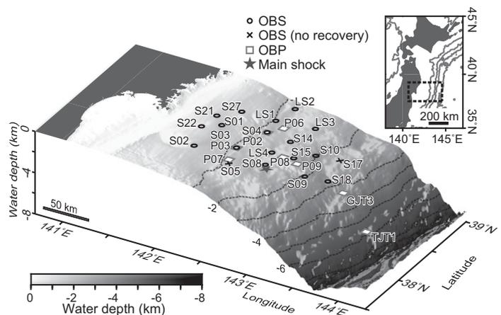
**Figure 1.** Locations of ocean-bottom pressure recorders (OBPs) and ocean-bottom seismometers (OBSs) off Miyagi, Tohoku region, north-eastern Japan. Seafloor map is from J-EGG500 (JODC-Expert Grid data for Geography-500 m; [http://www.jodc.go.jp/data\\_set/jodc/jegg\\_intro.html](http://www.jodc.go.jp/data_set/jodc/jegg_intro.html)). Star indicates epicenter of main shock on 11 March 2011.
