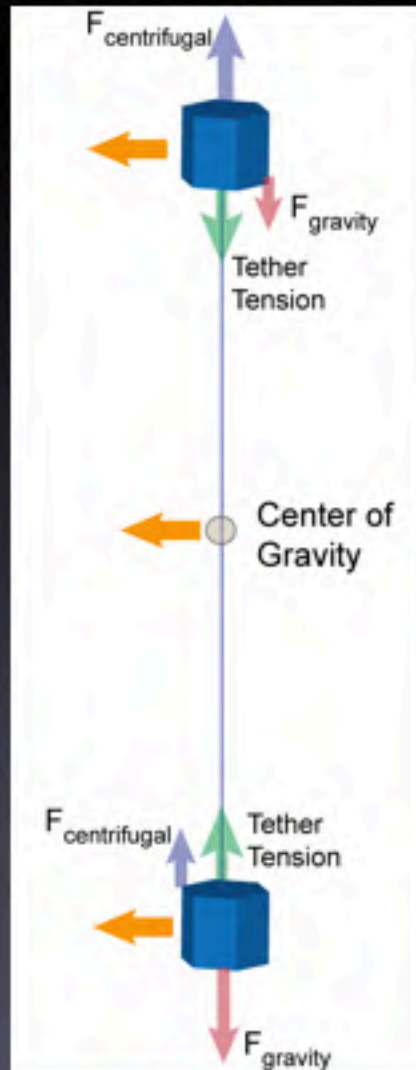
Tether forces satellites to co- orbit at center of gravity's orbital velocity
