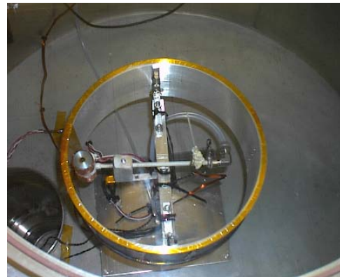
Figure 2. Photo of the dipole and plasma source system inside the vacuum chamber
