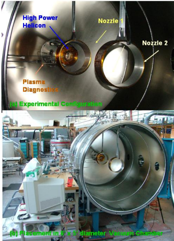
Figure 10. (a) Interior view of the placement of the high power helicon and magnetic nozzles, and (b) exterior view of the experimental setup including the vacuum chamber.
